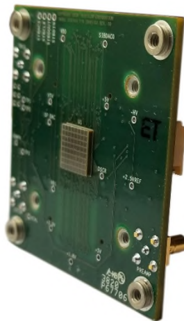
Figure 3: S13615-1025N-08 Detector Mounting
