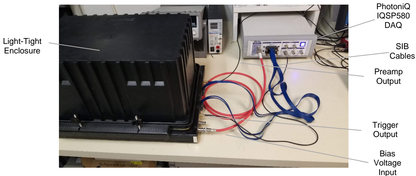
Light-Tight Enclosure (Electrical Connections)
